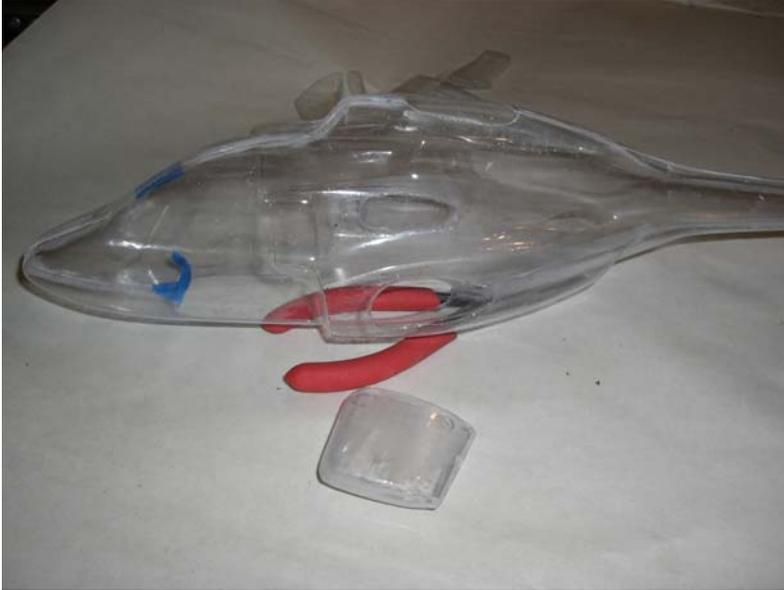
For the Airwolf build you have 2 options for installing the wheel wings. First option is to use the short wings and glue them right to the surface. The 2<sup>nd</sup> option is to trim out the sunken wing area and insert the full size wings from the inside. The wings will actually pop in place when inserted far enough. If you use the 2<sup>nd</sup> option you can trim down the smaller ones to use as gun covers if you build exposed machine guns.
