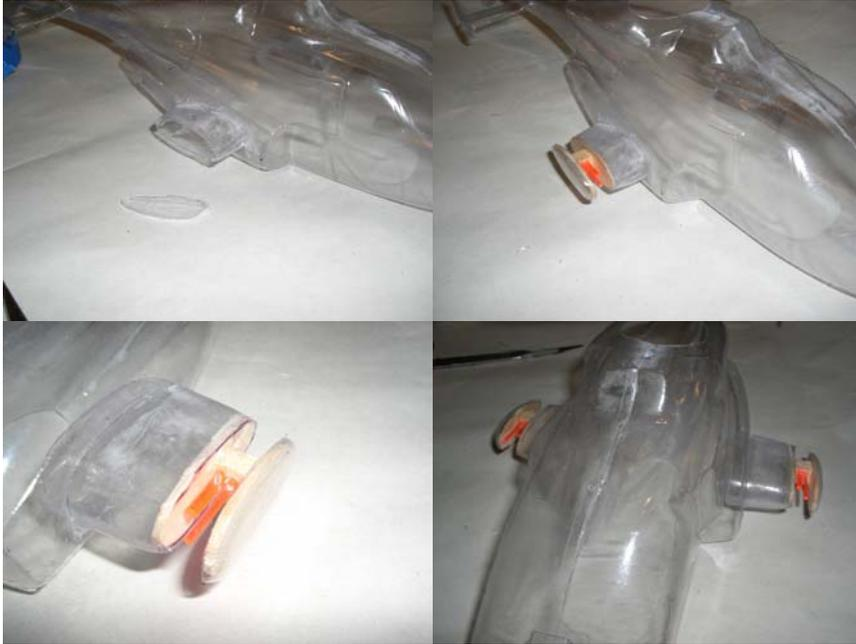
Wash the fuselage with mild soap and water before masking and painting. I usually paint before installing the landing gear or engine exhaust. Install the landing gear as shown in the following pictures.
