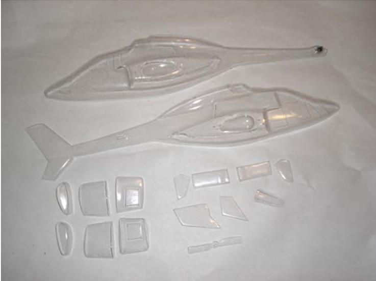
Fit the 2 sides of the fuselage trimming as needed. When you have a good fit use masking tape to hold the sides together. Glue with your choice of glues I use CA but epoxy also works well. Make sure you avoid the window areas with the glue.
